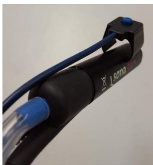
Figure 3B: Monopolar Handswitch Housing Connection
