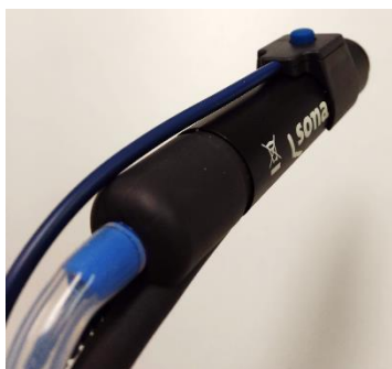
Figure 3B: Monopolar Handswitch Housing Connection
