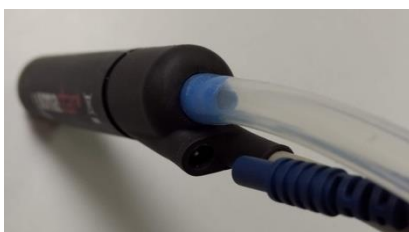
Figure 3A: Monopolar Handswitch Handpiece Cable Connection
