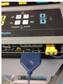
Figure 2C: Monopolar Handswitch Electrosurgical Cable Connection
