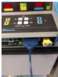
Figure 2C: Monopolar Handswitch Electrosurgical Cable Connection
