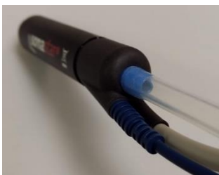
Figure 3A: Monopolar Handswitch Handpiece Cable Connection
